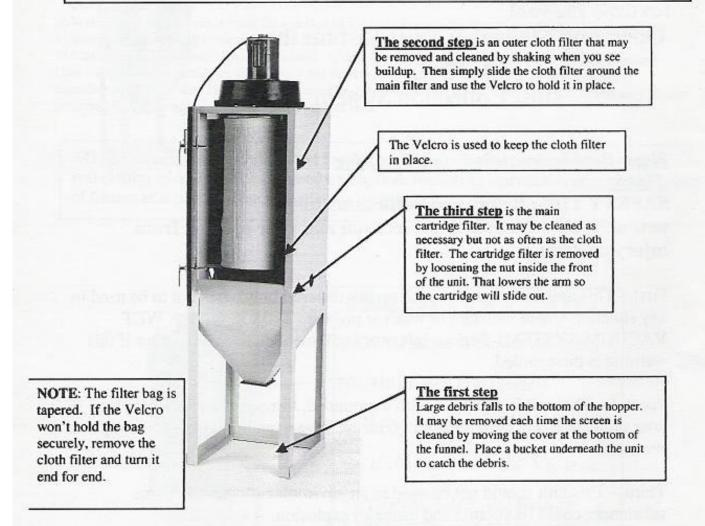
Note: Failure to clean the filter system may cause damage to the motor and cartridge filter. These are expensive replacement items. The outer cloth filter may need replacement and may be purchased from Cyclone Manufacturing Inc. The first stage screen should last indefinitely.
